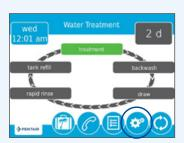
a At your softener, press the **Gear icon** on the display. Press the Bluetooth<sup>®</sup> wireless technology Off button then use the right arrow to turn Bluetooth on (also make sure your phone's Bluetooth<sup>®</sup> is on).
