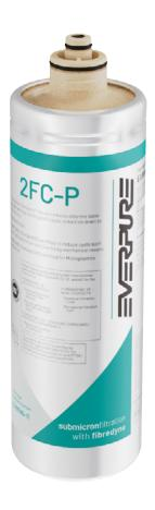
The 2FC-P water filtration cartridge featuring exclusive Fibredyne™ media is designed to reduce PFOA/PFOS, chlorine, taste & odor, lead, microplastics and particulates. These features can help ensure reliable, long-lasting equipment performance. The system using this cartridge can maintain a flow rate of 5.69 l/min for over 3″750 liters.
