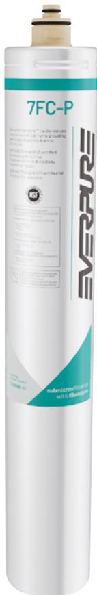
The 7FC-P water filtration cartridge featuring exclusive Fibredyne™ media is designed to reduce PFOA/PFOS, chlorine, taste & odor, microplastics and particulates. These features can help ensure reliable, long-lasting equipment performance. The system using this cartridge can maintain a flow rate of 6.32 l/min for over 37'800 liters.
